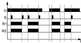
On occurrence of a pulse on the control input S, output relays R1 and R2 are switched on. This status lasts until another control pulse occurs - then, the output relays R1 and R2 are switched off.
