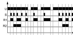
When a pulse occurs on the control input S, the output relay R1 is switched on. The status lasts until another control pulse occurs - then, the output relay R1 is switched off, and the R2 relay is switched on.
