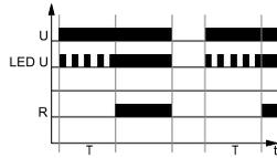
When the supply voltage U is applied, the set interval T begins (green LED flashes). After the interval T has expired (green LED illuminated) the output relay R switches into on-position (yellow LED illuminated). This status remains until the supply voltage is interrupted. If the supply voltage is interrupted before the expiry of the interval T, the interval already expired is erased and is restarted when the supply voltage is next applied.
