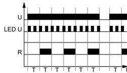
When the supply voltage U is applied, the set interval T begins (green LED flashes). After the interval T has expired, the output relay R switches into on-position (yellow LED illuminated) and the set interval T begins again. After the interval T has expired, the output relay switches into off-position (yellow LED not illuminated). The output relay is triggered at a ratio of 1:1 until the supply voltage is interrupted.
