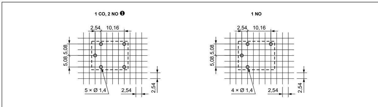
① Set of two normally open contacts with a common connection for the moving contact. ② In case of no tolerance shown in outline dimensions: outline dimension  $\leq 1$  mm tolerance should be  $\pm 0,2$  mm;  $> 1$  mm and  $\leq 5$  mm tolerance  $\pm 0,3$  mm;  $> 5$  mm tolerance  $\pm 0,4$  mm.
