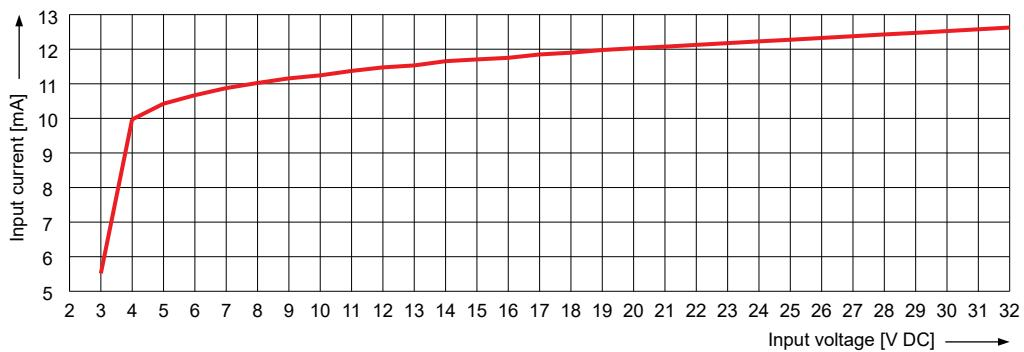
③ The input curve is measured at ambient temperature 25 °C.
