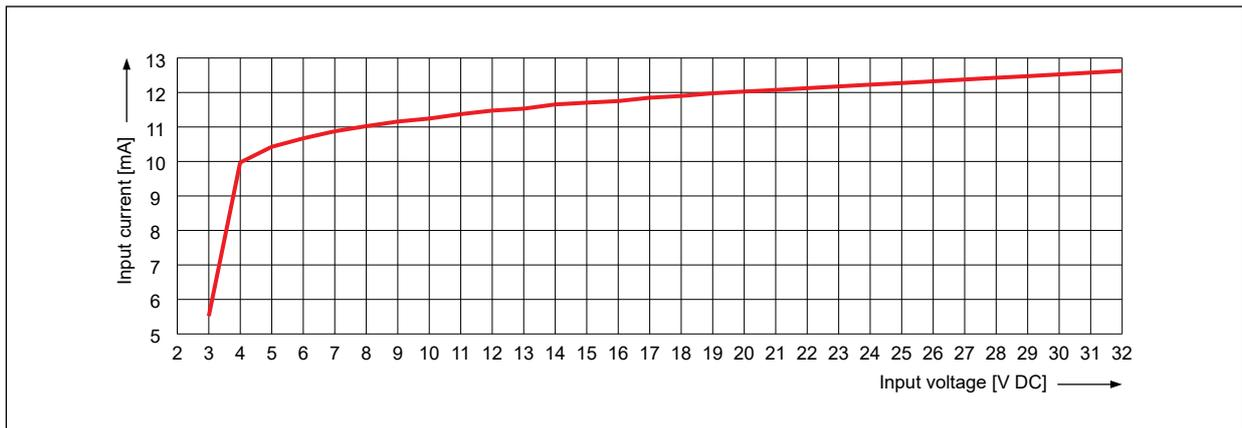
⊗ The input curve is measured at ambient temperature 25 °C.
